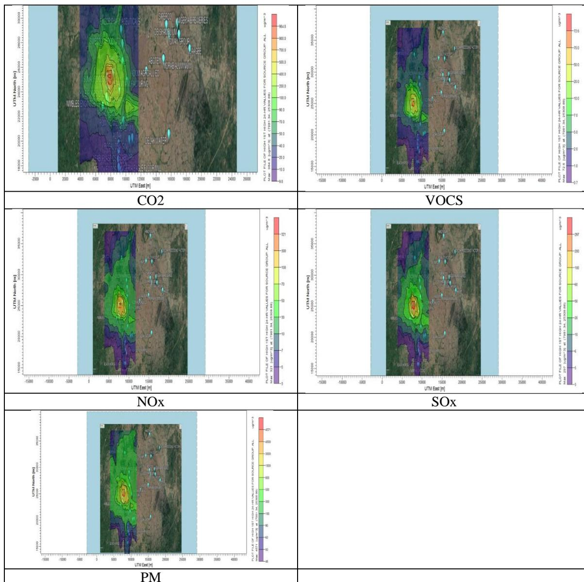
Fig.4 Predicted ground level concentration of Carbon monoxide (CO), Volatile Organic Compound (VOC), Particulate Matter (PM), Sulphur Oxide (SO<sub>x</sub>) and Nitrogen Oxide (NO<sub>x</sub>) respectively.
