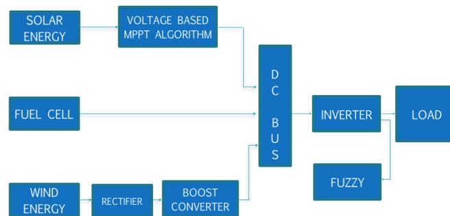
**Fig 4.1** Block diagram of hybrid system
