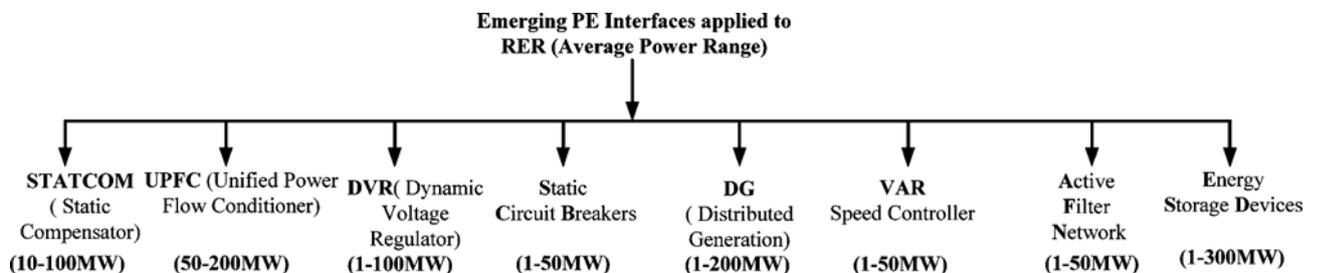
Fig. 2.3. Different applications of PE with respect to RER
