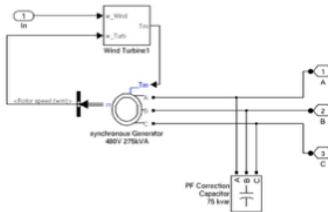
Fig 3.2.3 Simulation for wind mill
