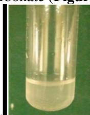
**Figure 11 : Turbidity shows the presence of Calcium Carbonate**
