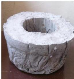
**Fig 31 : Small well constructed using Cement and Biobricks**
