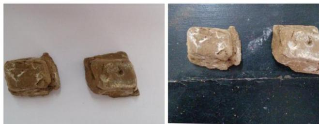
Figure 17 : Calcium Carbonate precipitation over the bricks
