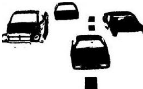
Figure 20 Edge detected and Flood Filled Image with vehicle converted from grayscale
